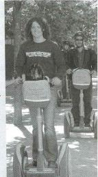
wheels and is guided by gyroscopes that respond to the body's movements. The rider stands on a small platform between the two wheels holding on to handlebars at waist height. It takes a while to get used to a Segway's movement, but once you do, it's a safe and comfortable way of getting around.
